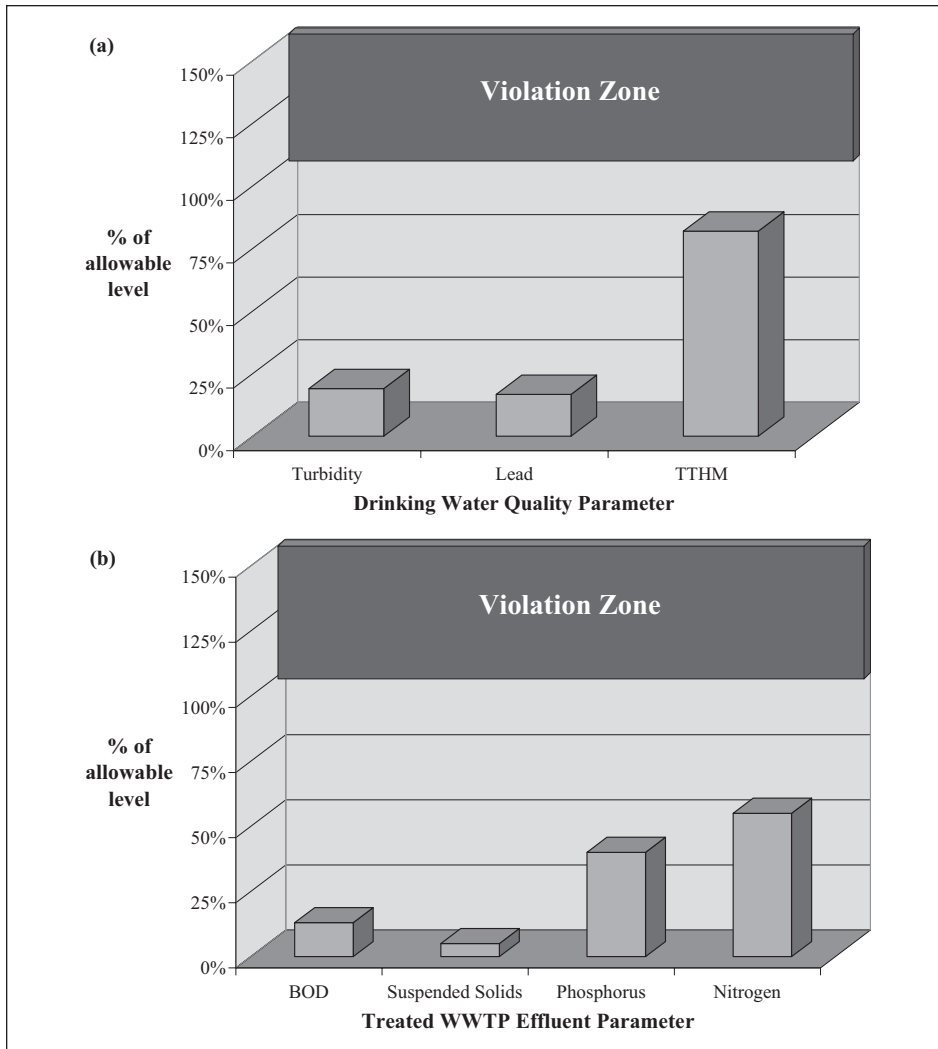
FIGURE 1 a. Drinking water quality. b. Treated wastewater effluent quality for calendar year 2010. TTHMs = total trihalo-methanes. BOD = biological oxygen demand. Source: WSSC.
